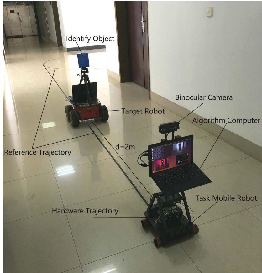
Figure 6: Experimental environment of the practical mobile robot, where a task mobile robot was tracing a target robot moving along a reference trajectory with a random changing velocity.
