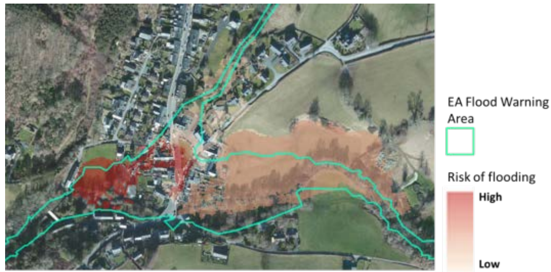
Figure 6: Figure 6: Using a DTM in conjunction with data captured by NOAH and the rolling ball technique, the likelihood of flooding is predicted and compared with the authoritative flood warning area as identified by the Environmental Agency (EA).
