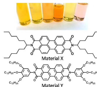
Figure 1; schematics of the chemical structures of the perylene-diimides (PDIs) being studied, denoted as materials X and Y as indicated. The clear solvatochromism of PDIs is shown (top inset), as material X is dissolved in a range of differing solvents.
