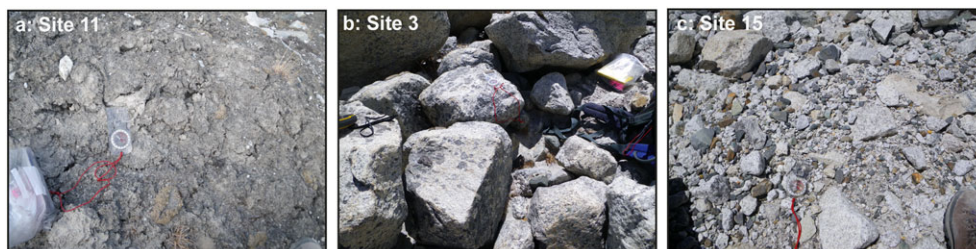
Figure 2. Site photos before installation of temperature sensors: (a) Site 11: consolidated medium sand with medium pebbles; (b) Site 3: small cobbles to large boulders with a medium to coarse sand matrix; and (c) Site 15: small granite and schist cobbles to small boulders with coarse sand to medium pebble matrix. [Colour figure can be viewed at wileyonlinelibrary.com ]
