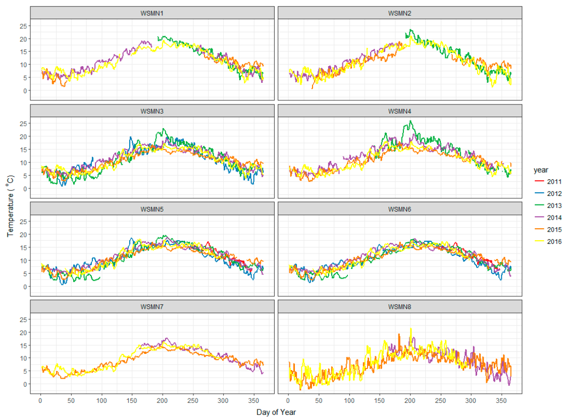
Figure 3. Time series of ST at 5 cm depth from the soil surface layer measured at the WSMN experimental sites from their individual installation dates to the present.
