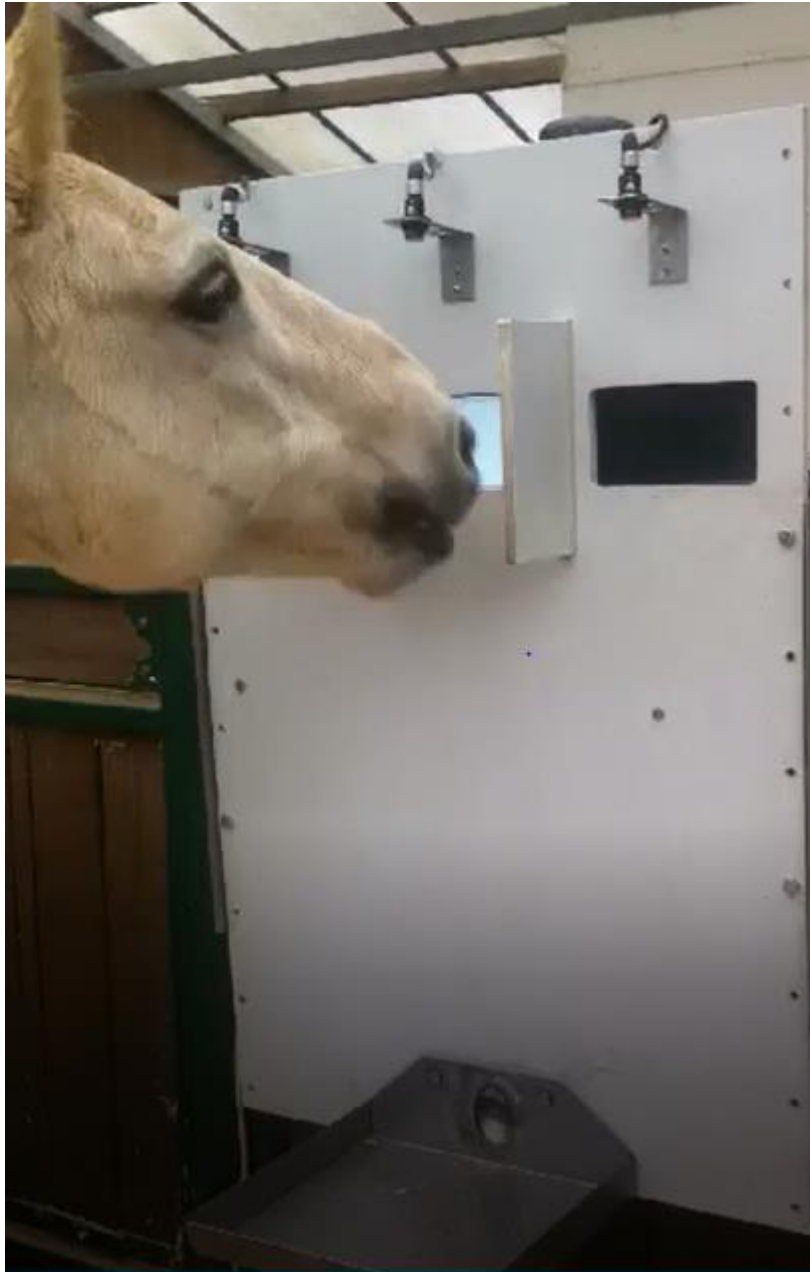
Plate 1. Performing the 3-CSRTT. NB image for demonstration purposes only, under experimental conditions the human is located to the immediate right hand side of the OS as to be unaware of CS presentations.
