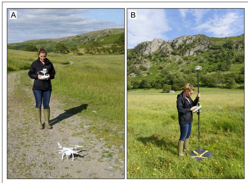
Figure 2 Fieldwork procedure for students to acquire aerial images: (A) RTK-GPS survey of a ground target; (B) Operation of the remote control for a DJI Phantom UAV. Note that these photographs were taken during undergraduate fieldwork in the UK rather than during the New Zealand fieldtrip but they illustrate the same procedure.
