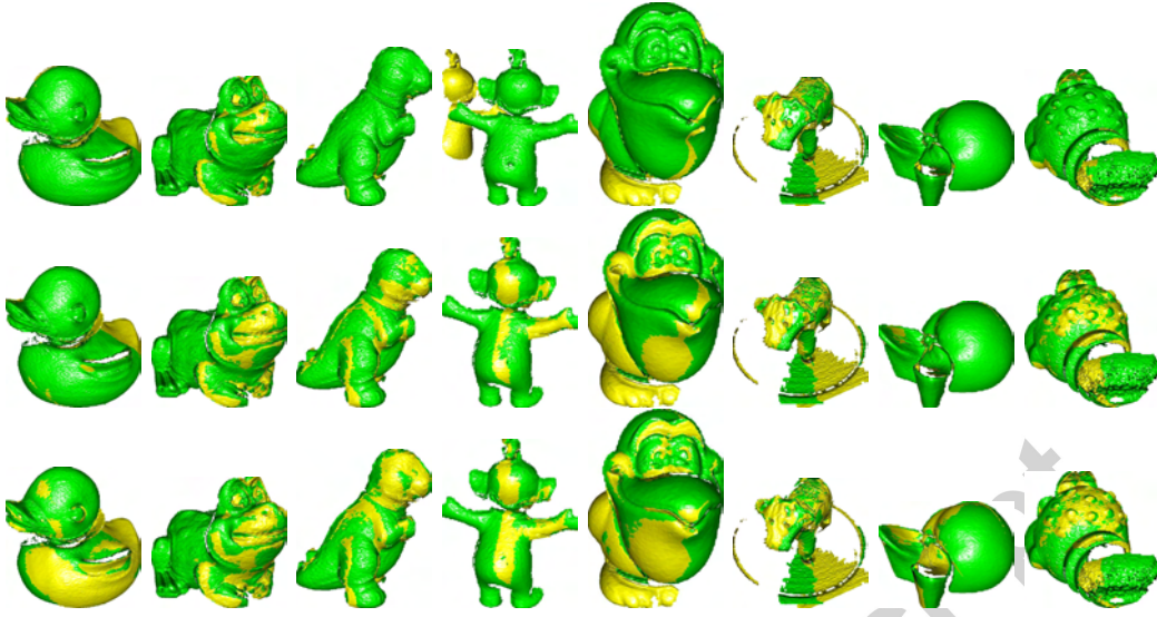
Figure 6: Final registration results for our RBAB method using different schemes for the fusion of the underlying transformations estimated by different weak estimators. From left to right: duck0–40, frog40–80, dinosaur144–180, tubby120–160, bird100–60, cow42–45, peach280–240, and lobster60–80. Top row: Complete; Middle: Partial; Bottom: Last solution.
