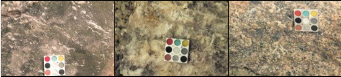
Figure 9. Close up images of polyhalite (left), halite (center) and sylvinite (right) taken under white light. CLUPI Calibration Target measures 2.5 x 2.5 cm 2 .
