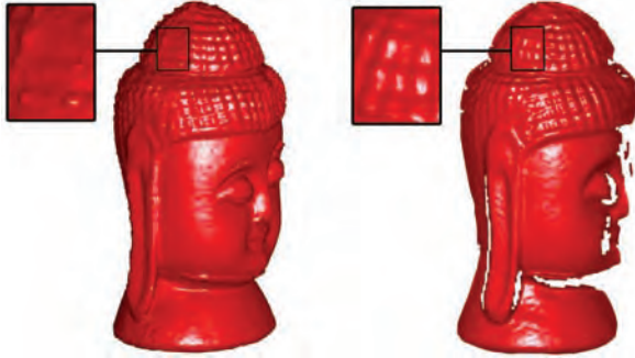
Figure 24: The limitation of our method. Although the proposed method is more robust to registration error than other methods, it fails to retain surface details when the registration error is excessively large. Left: the integration of 18 Buddha scans produced by our method. Right: one input scan used as the ground truth
