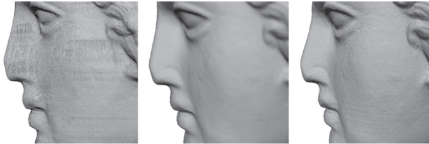
Figure 19: Integration results of the mask scans. Left: without integration; Middle: pairwise MRF-based integration [22]; Right: our integration
