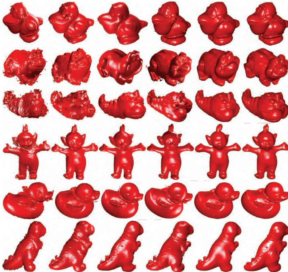
Figure 12: Rows: Integration results of 17 Bird scans, 17 Frog scans, 18 Lobster scans, 17 Teletubby scans, 18 Duck scans and 11 Dinosaur scans. From left to right: volumetric method[12], mesh-based method[18], SFK[16], k-means[15], pairwise MRF[22], our method
