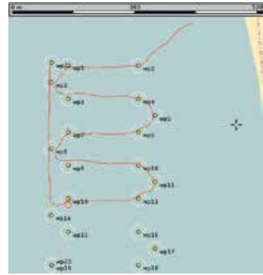
Figure 10: A map showing a survey pattern being followed using the cross track error minimization controller. The white circles around each waypoint indicate the threshold distance and the red line indicates the path taken.
