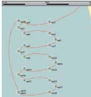
Figure 9: A map showing a survey pattern being followed using only a heading controller. The white circles around each waypoint indicate the threshold distance and the red line indicates the path taken.
