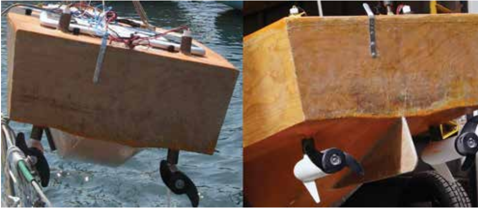
Figure 6: The hull before and after the skeg was attached.
