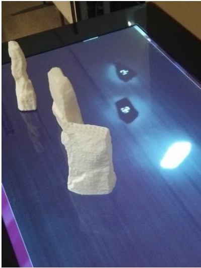
Fig. 15. Tangible models on the Samsung SUR40 multi-touch table: the black foam bases absorb the excess infrared light and highlight the byte tag.
