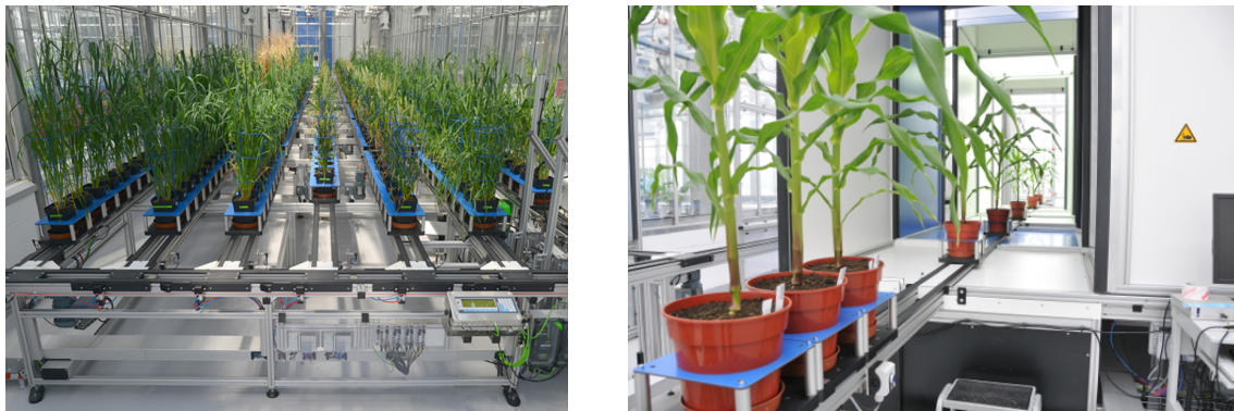
Fig. 1 The UK NPPC. Left, One of the robotic greenhouses; Right, Plants (here, maize) entering the imaging chambers.
