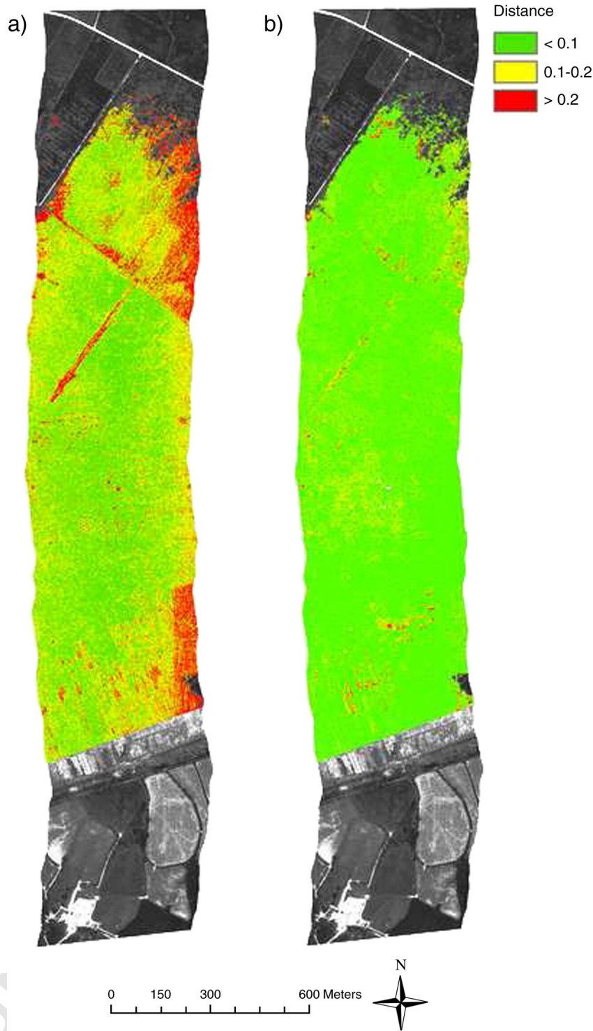
Fig. 9. Map of Euclidean distances between mapped pixels and the nearest-neighbour field sampling plot in Isomap space for a) species level data and b) plant functional type (PFT) data. Green values indicate that a pixel's reflectance is similar to a sampled plot, whereas red pixels indicate the greatest dissimilarities between the image and plot samples and thus indicate greater uncertainty in the model. A normalised difference vegetation index image is used as the background image. (For interpretation of the references to color in this figure legend, the reader is referred to the web version of this article.)
