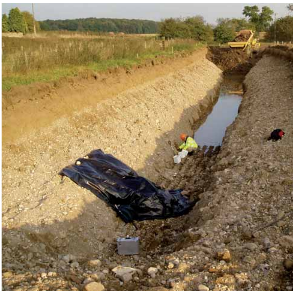
Fig 31 Sampling fluvial gravels near Ripon, Yorkshire: a black plastic tarpaulin was used to exclude light and the sample was collected in a thick black plastic bag (photograph by G A T Duller).
