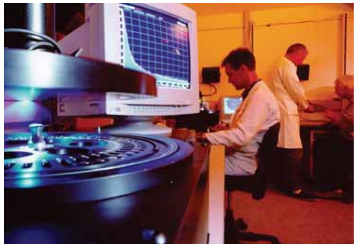
Fig 6 (left) Typical OSL signal observed from a quartz aliquot – the OSL signal drops rapidly as the trapped electrons in the quartz are used up to produce the luminescence signal. (right) An automated luminescence reader equipped with blue-light-emitting diodes (LEDs). When in use, the lid closes, leaving the sample holder in darkness. The blue LEDs are switched on to measure the optically stimulated luminescence (OSL) signal (© Risø National Laboratory, Denmark).
