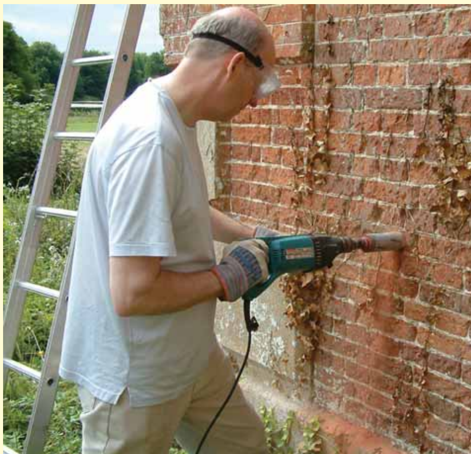
Fig 40 Using a diamond tipped drill barrel to sample a brick for OSL dating.
