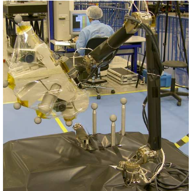
Figure 4: Calibration setup with the Beagle2 Flight Model (FM) ARM and 1/3rd mass PAW in Astrium Ltd. clean room.
