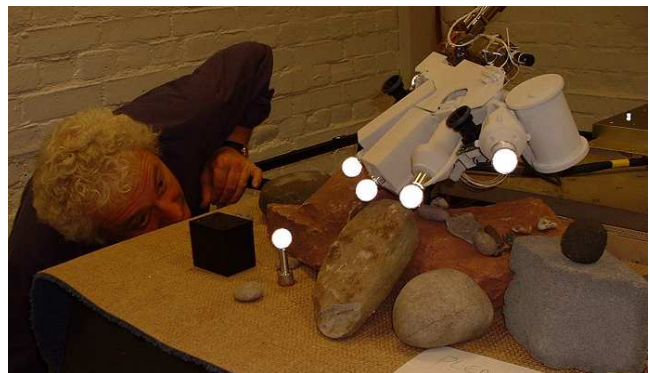
Figure 10: DM ARM and 1/3rd mass PAW tests using virtual ARM/PAW model, and mock terrain.
