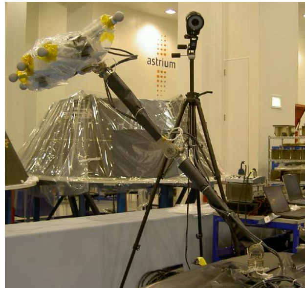
Figure 6: Beagle2 FM ARM and 1/3rd mass PAW in Zero PAW State position.
