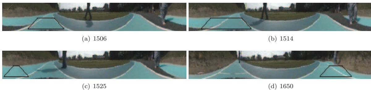
Figure 29: Failure case of the RGB colour space on the RUNNINGTRACK dataset: the detection moves onto a joining track on the left and then moves on the back of the robot
