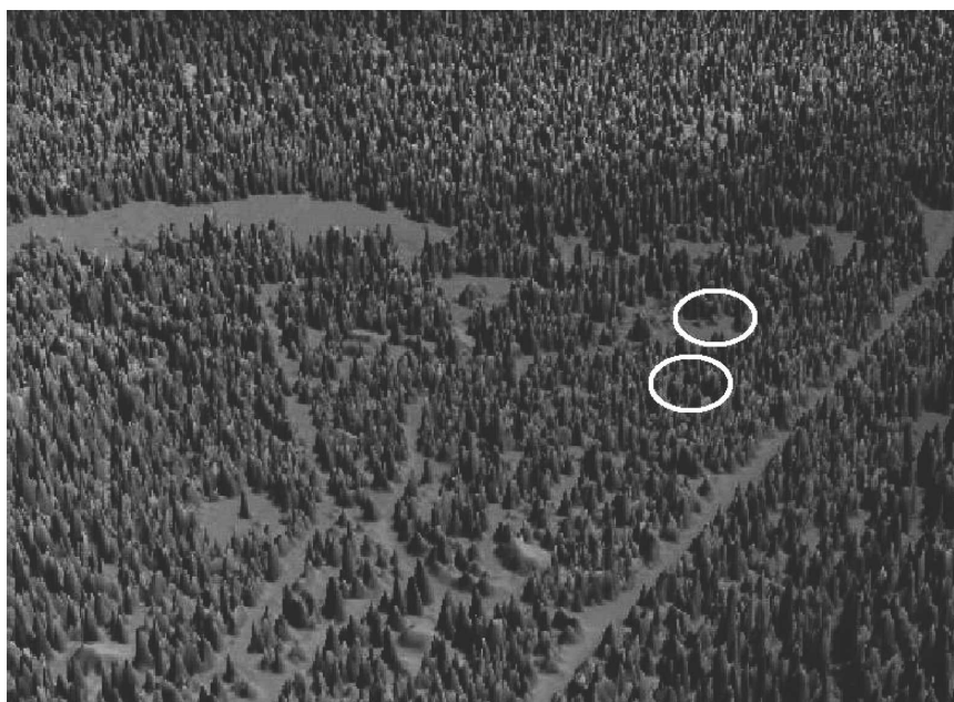
FIG. 1. Rendered representation of the lidar first return of the Fraser pine forest showing the locations of the discontinuous (upper circled area) and uniform (lower circled area) stands.
