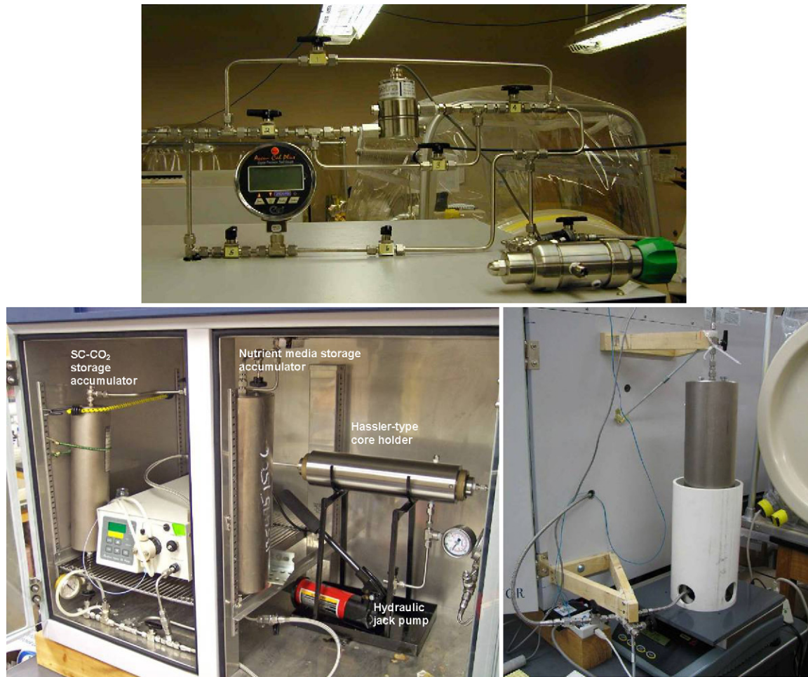
Fig. 3 – Pictures of high-pressure biofilm and supercritical CO 2 flow system: top—series of valves and gauges that allow differential pressure to be controlled. Bottom left: Nutrient media accumulator, supercritical CO 2 storage accumulator, Hassler-type core holder containing Berea sandstone core, and hydraulic jack pump used to apply overburden pressure. All housed inside an incubator for temperature control. Bottom right: Accumulator and sample port used to collect effluent samples.
