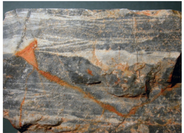
Figure 4: Example rock face demonstrating lamination features (Pullan, 2007)
