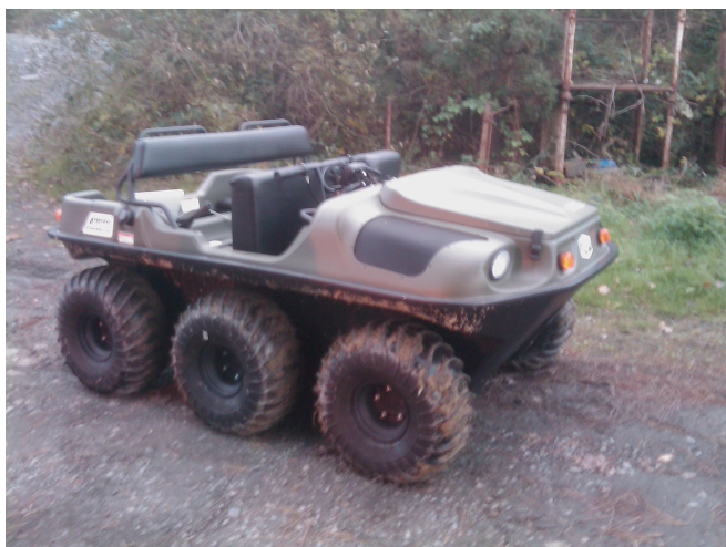
Fig. 1. The ARGO 6x6 Frontier 580 Amphibious Skid-Steer Vehicle
