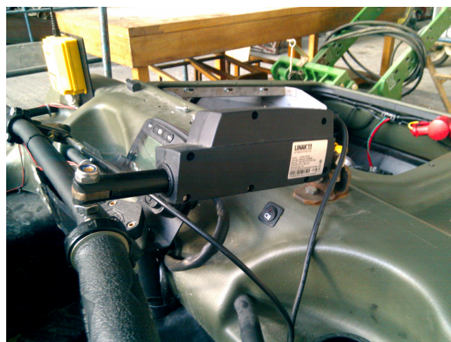
Fig. 3. The LINKAK LA12 linear actuator bolted to the ARGO handlebars allowing for their manipulation via computer.
