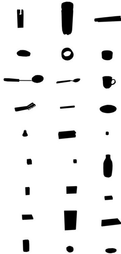
Fig. 5: The selection of object images used to train the affordance learning memory with. These were taken from human grasp experiments and therefore each come with the accompanying synergy values required to grasp them.
