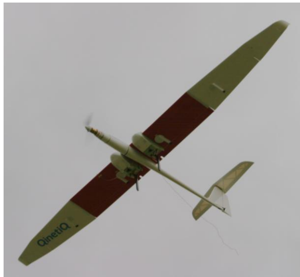
Figure 1. Underside view of the UAV showing camera pods.
