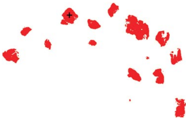
Figure 12. Plan view of “rock garden” DEM data that have been processed to obtain the rock planar regions for arm placement purposes. The black crosshair denotes the centroid on the largest contiguous planar region.
