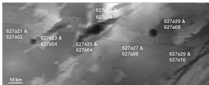
Figure 7. Digital elevation model of part of Mareotis Fossae. The whole area is covered by the MOLA digital elevation model. The lighter part of the DEM emphasizes the area where Viking stereo coverage (used image numbers shown) has improved the resolution of the MOLA digital elevation model. For this area, DN height resolution is 15 m.
