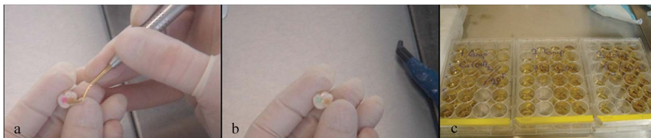
Figure 2. Sealing of cavities in different coloured compomer materials (a, b); tooth samples placed inside microplates for further evaluation (c).
