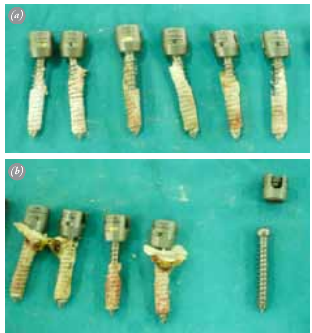
Fig. 3. (a) View of the CAS-augmented screws after pull-out test. All the thread of the screw is coated with calcium sulfate cement. (b) View of the PMMA-augmented screws after pull-out test. Polyaxial head breaking off was observed during testing procedure in a screw. [Color figure can be viewed in the online issue, which is available at www.aott.org.tr ]
