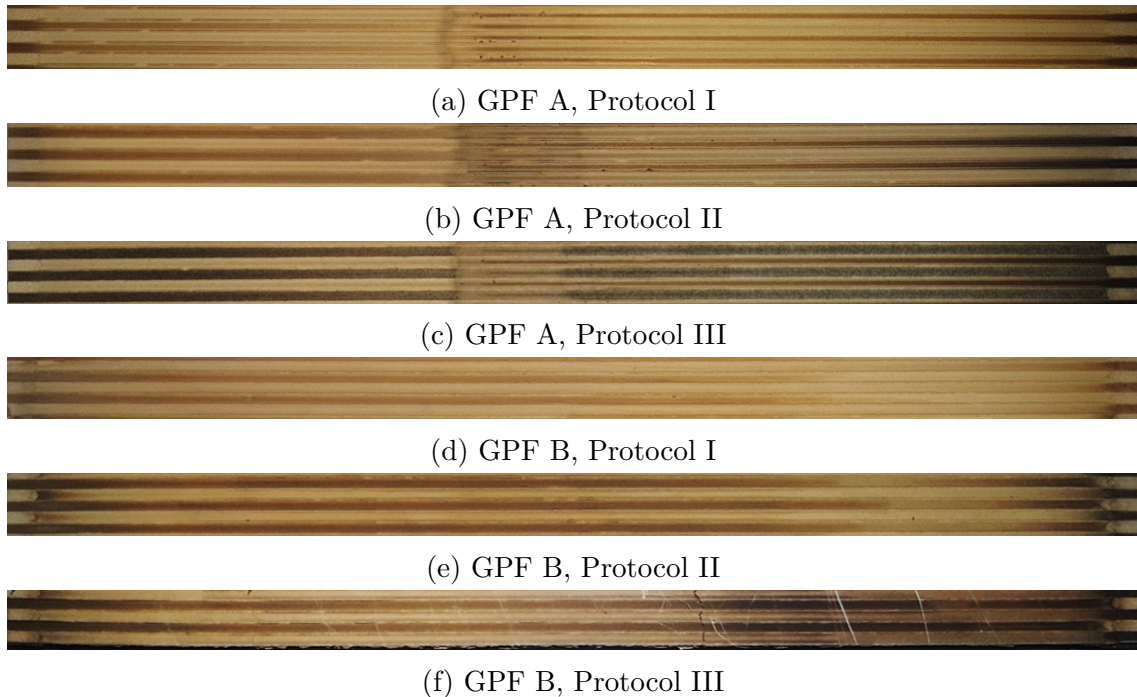
Fig. 8.5: Axial photographs of GPF (a-c) A and (d-f) B after each soot loading protocol. The brightness and contrast have been increased for clarity. The white marks in (f) are strands of PTFE tape that remained after the sample was unwrapped following the MRI experiments.
