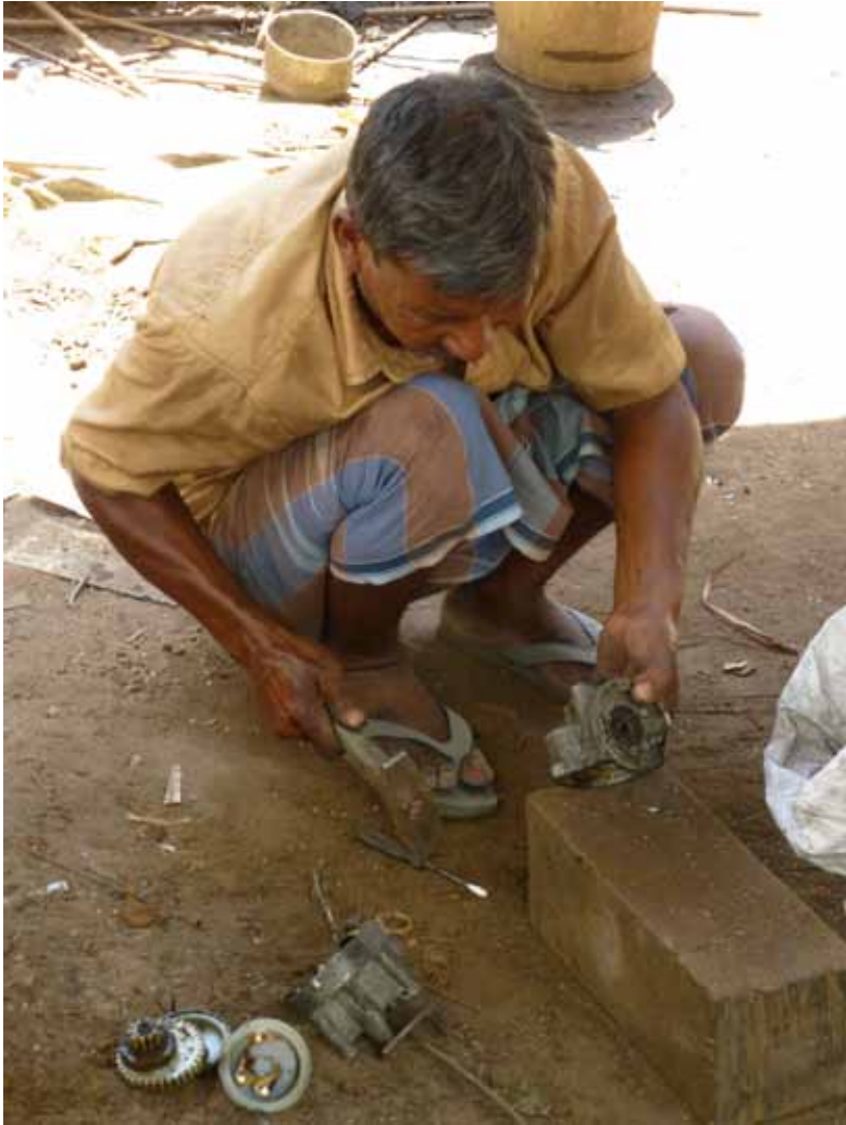
FIGURE 2: Disassembling an electrical motor. Photograph © Andrew Sanchez
