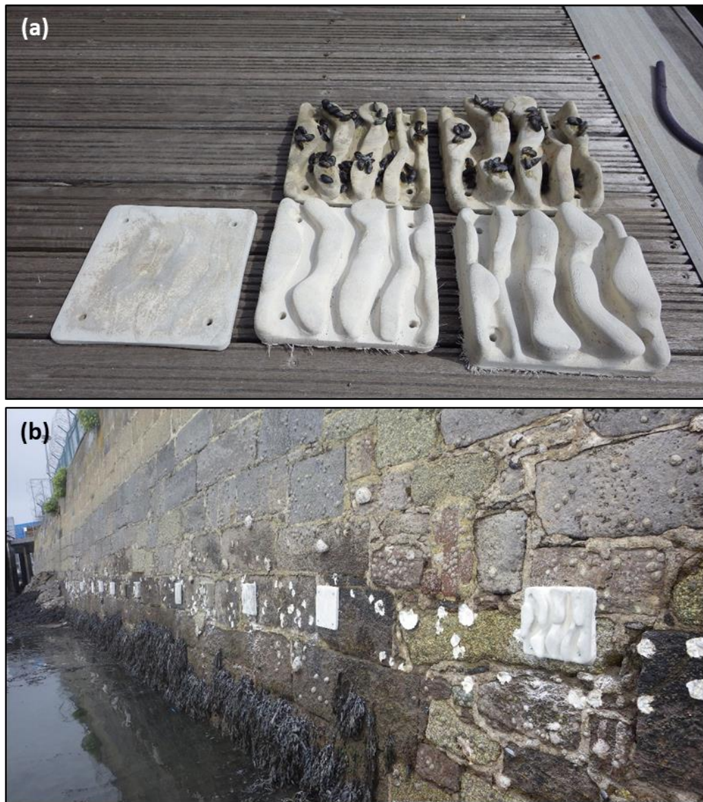
Figure 4-2. Eco-friendly experimental tiles (a) showing the flat, 2.5 cm and 5 cm complexity treatments (from left to right), with tiles seeded with mussels shown above, and (b) attached to the seawall at Turnchapel Wharf, Plymouth, British Isles.
