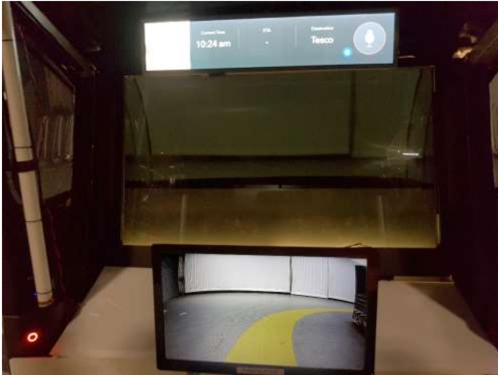
Figure 6 – Camera Feed interface showing live footage of the road ahead and the intended path in yellow. Hazards would also be shown in orange rectangles.
