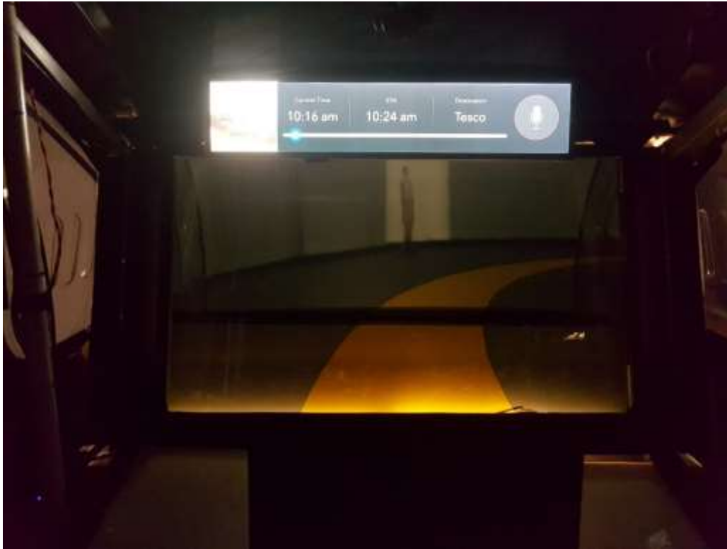
Figure 7 – Augmented reality (AR) heads-up display semi-transparent screen showing hazards in the environment (highlighted rectangle) and the intended path (yellow stripe)
