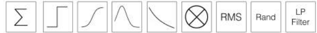
Figure 1. Graphical symbols used for the schematic representation of network nodes and connections. From left to right: summation, threshold function, sigmoid transfer function, gaussian transfer function, negative exponential function, gain function, root mean square (RMS), random number generator, low pass filter.
