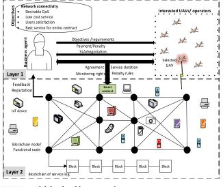
FIGURE 2. High level architecture environment.
