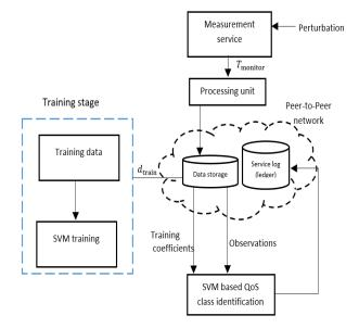
FIGURE 4. Flow diagram of QoS monitoring.
