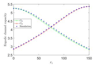
**FIGURE 6.** Comparison between simulation and theoretical results for ergodic capacity as a function of  $r_i$ , when  $P_D^{d_i-r_i} = P_{E_i}^{r_i} = -77.12$ dBm.
