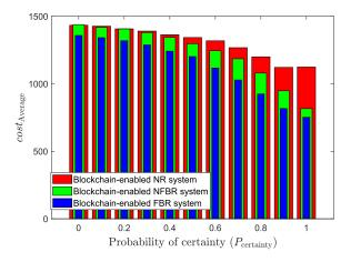
**FIGURE 9.** Performance comparison between the proposed blockchain-enabled FBR system and NFBR and NR systems in terms of the total service cost as a function of certainty, when the number of monitoring nodes is 10,  $\kappa = 0.5$ , and  $n_u = 50$  (number of UAV operators).
