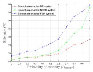
**FIGURE 10.** Percentage efficiency of blockchain-enabled FBR, NFBR and NR systems as a function of probability of certainty, when the number of monitoring nodes is 10,  $\kappa = 0.5$ , and  $n_u = 50$ .
