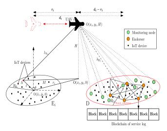
**FIGURE 1.** A UAV located at  $O(x_i, y_i, H)$  intends to serve two pockets of areas - region  $E_i$  of its existing service area and region D of new service area in order to earn profit out of its extra resources.
