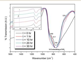
Fig. 6 IR spectra of batched β-Pb<sub>3</sub>(VO<sub>4</sub>)<sub>2</sub> and Pdl<sub>2</sub> subjected to HEBM after  $t=0,\,1,\,10,\,20,\,$  and 30 h. Inset: stacked IR spectra showing amorphisation of V–O stretching in the VO<sub>4</sub> unit as a function of HEBM time.
