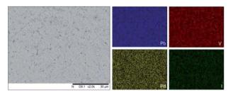
Fig. 12 BSE SEM image at  $\times$  2000 magnification (scale bar length = 30  $\mu$ m) and EDX map of Pb (blue), V (red), Pd (yellow), and I (green) present in "PdPb<sub>9</sub>(VO<sub>4</sub>)<sub>6</sub>I<sub>2</sub>" HEBM reacted at 200 °C for 1 h in a sealed quartz tube. EDX spectra are shown in Fig. S2.†
