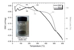
Fig. 9 DSC (black line) and TGA (grey line) curves from 30 to 600 °C under flowing Ar(g) of "PdPb<sub>9</sub>(VO<sub>4</sub>) $_6$ l<sub>2</sub>" batched powders after 30 h HEBM. Insert: resulting powder after 30 h HEBM.
