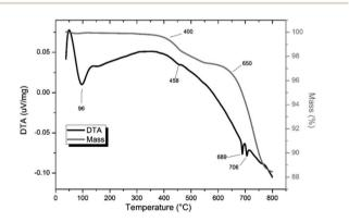
Fig. 4  $\,$  TGA-DTA analysis of "PdPb9(VO4)6I2" reacted in a sealed vessel under vacuum at 500  $^{\circ}C$  for 5 h.
