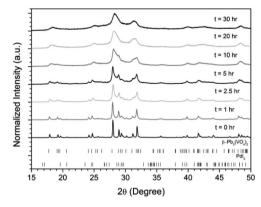
Fig. 5 PXRD patterns of batched  $\beta$ -Pb<sub>3</sub>(VO<sub>4</sub>)<sub>2</sub> and Pdl<sub>2</sub> subjected to HEBM after t=0, 1, 2.5, 5, 10, 20, and 30 h. Respective tick marks represent allowed reflections for  $\beta$ -Pb<sub>3</sub>(VO<sub>4</sub>)<sub>2</sub> (ICSD 1008164; top ticks) and Pdl<sub>2</sub> (ICSD 1539344; bottom ticks).
