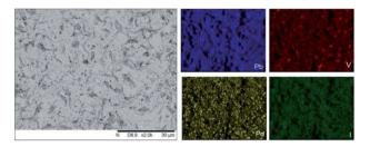
Fig. 13 BSE SEM image at  $\times 2000$  magnification (scale bar length =30  $\mu m)$  and EDX map of Pb (blue), V (red), Pd (yellow), and I (green) present in "PdPb9(VO4)6[2" HEBM reacted at 500 °C for 1 h in a sealed quartz tube. EDX spectra are shown in Fig. S2.†
