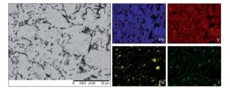
Fig. 2 BSE SEM image at  $\times 2000$  magnification (scale bar length =30  $\mu m)$  and EDX map of Pb (blue), V (red), Pd (yellow), and I (green) present in "PdPb9(VO<sub>4</sub>)<sub>6</sub>I<sub>2</sub>" reacted at 500 °C for 5 h in a sealed quartz tube. EDX spectra are shown in Fig. S2.†
