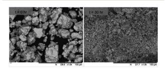
Fig. 8 SEM images ( $\times 1000$  magnification) showing particle size and morphology of initially batched powders (t=0) and after HEBM t=30 h. Scale bars shown at the bottom right of each image represent 100  $\mu$ m.
