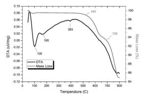
Fig. 14 TGA-DTA analysis of "PdPb9(VO4) $_6$ l2" subjected to HEBM 30 h and reacted at 500 °C for 1 h in a sealed vessel under vacuum.
