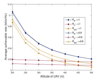
Fig. 8: The effects of the UAV altitude on the average rates, with  $P_{\rm U}=30$  dBm,  $\lambda_{\rm U}=100/{\rm km^2},~\lambda_{\rm E}=40/{\rm km^2},$  and  $N_{\rm R}=16.$
