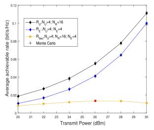
Fig. 5: The effects of the UAV transmit power on the average rates, with  $\lambda_{\rm U}=100/{\rm km^2},~\lambda_{\rm E}=300/{\rm km^2},~H_{\rm U}=300{\rm m},\rho=10{\rm m}.$
