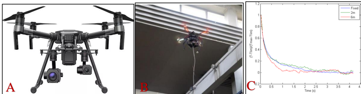
FIGURE 13 A: DJI M210 equipped with thermal camera [8]. FIGURE 13 B: UAV equipped with thermal camera [7]. FIGURE 13 C: Comparison of front face temperature responses to flash heating in the case of a large uniform irradiation with a fixed camera and a stabilized camera with UAV at two distances (2 m and 6 m) [7].
