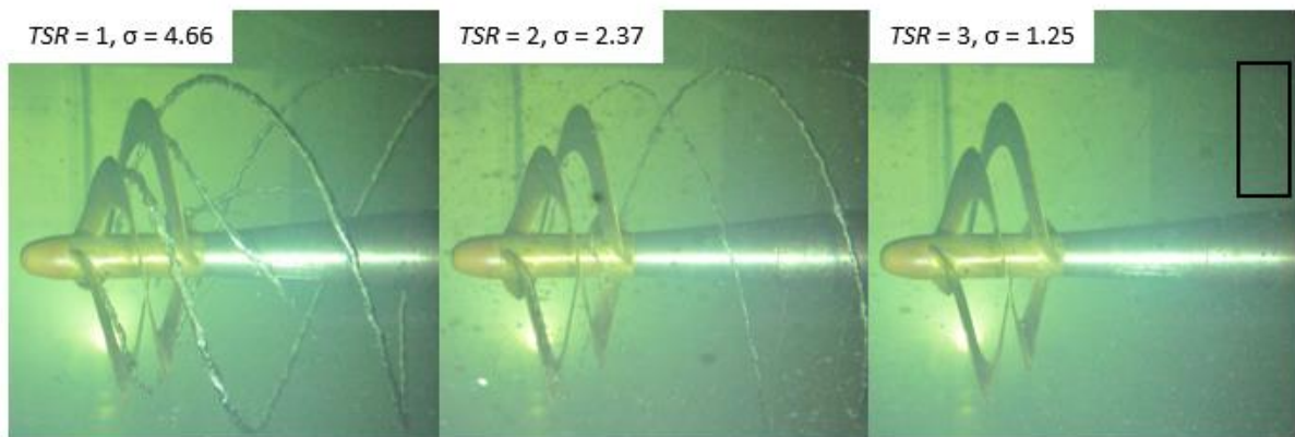
Fig. 9: Cavitation observation at high vacuum pressure
