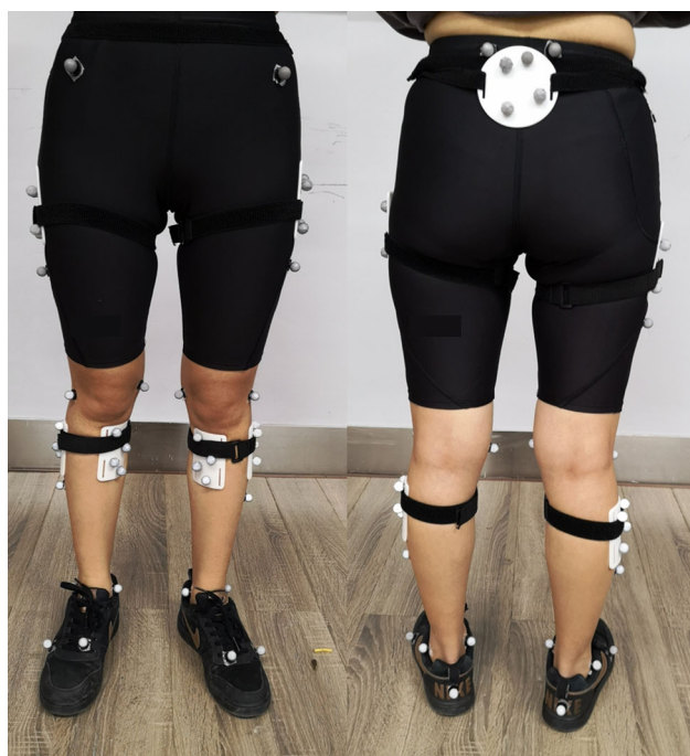
Figure 3. A combined marker set-up for the Strathclyde functional cluster model (SFCM), plug-in gait (PiG) and human body model gait (HBM2).
