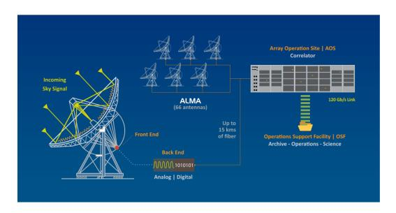
Figure 2.3: Signal processing using several radio telescopes).
