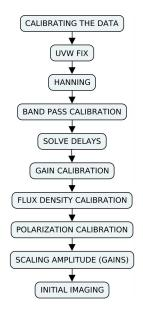
Figure 2.16: Main phases of the eMerlin pipeline.
