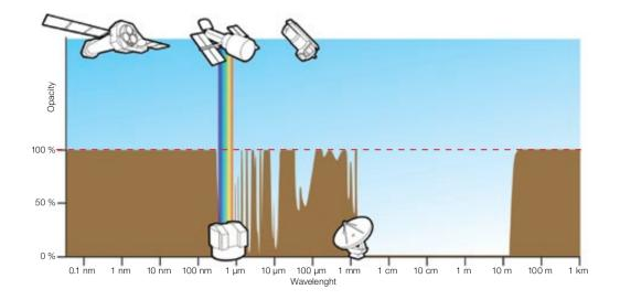
Figure 2.2: Atmospheric window (opacity generated by the atmosphere (percentage) v/s signal wavelength (m)).
