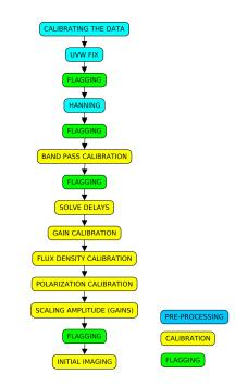
Figure 2.18: Stages of the eMerlin pipeline.
