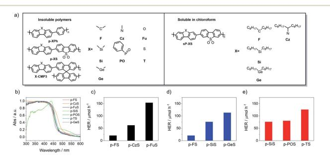
Fig. 1 (a) Structures of the polymer photocatalysts in this study; (b) UV/vis spectra of the 7 dibenzo[*b*,*d*]thiophene sulfone-containing photocatalysts, as measured in the solid state; hydrogen evolution rates of (c) **p-FS**, **p-CzS** and **p-FuS**; (d) **p-FS**, **p-SiS** and **p-GeS**; (e) **p-SiS**, **p-POS** and **p-TS** under visible-light irradiation ( $\lambda > 420$  nm, 300 W Xe light source).
