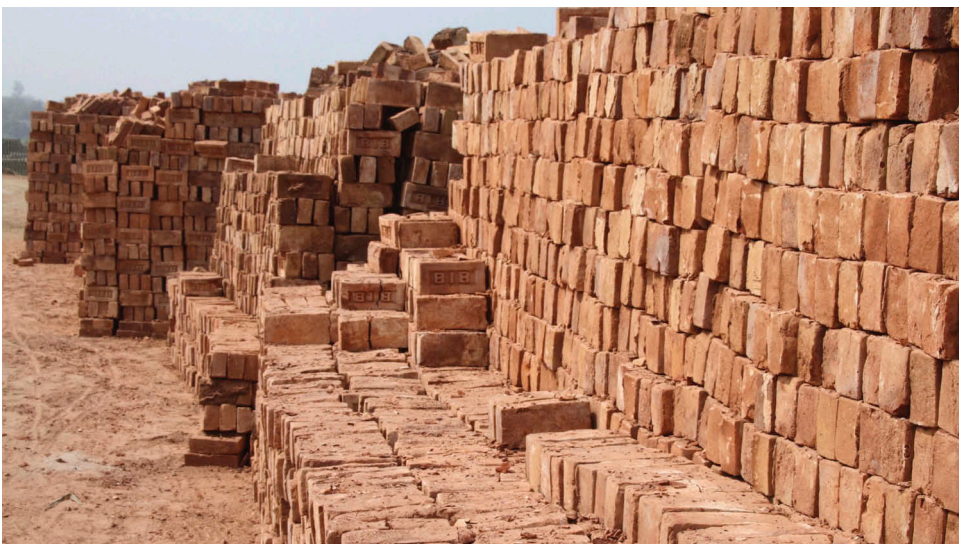
Figure 2. Piles of clay fired Bangla bricks. Credit: Author.
