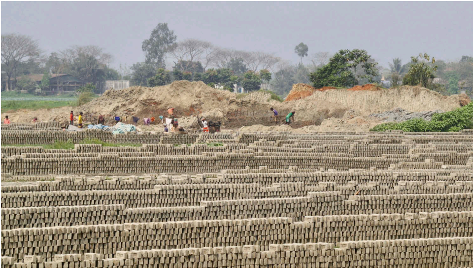
Figure 3. Soil preparation for brickmaking. Credit: Author.
