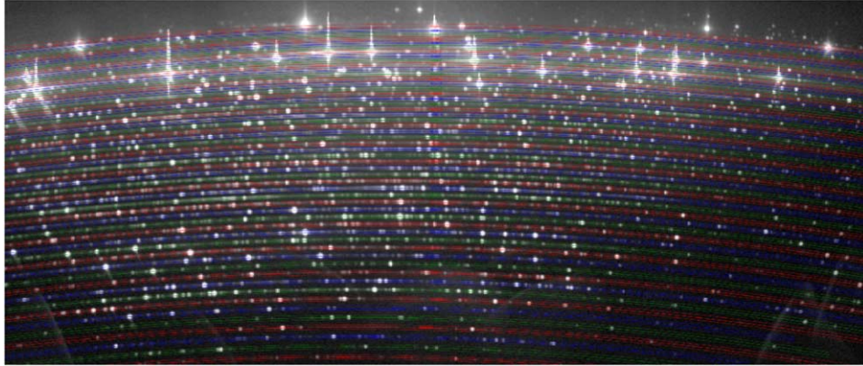
Figure 4. Images of a long-exposed Th–Ar spectrum taken with MRES. The brightness is scaled to logarithmic. The traces of the orders are shown (alternating red, blue, green).
