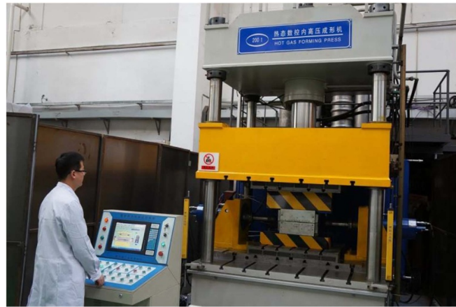
Figure 22. A 70 MPa HGPF platform developed by Harbin Institute of Technology.
