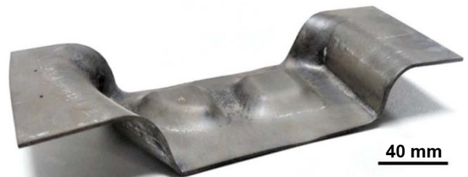
Figure 31. TC4 titanium alloy wing stiffener formed by hot stamping.
