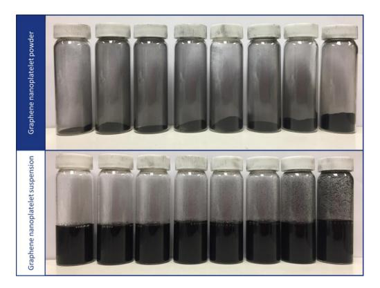
Figure 1. Top: Graphene nanoplatelet powders.
