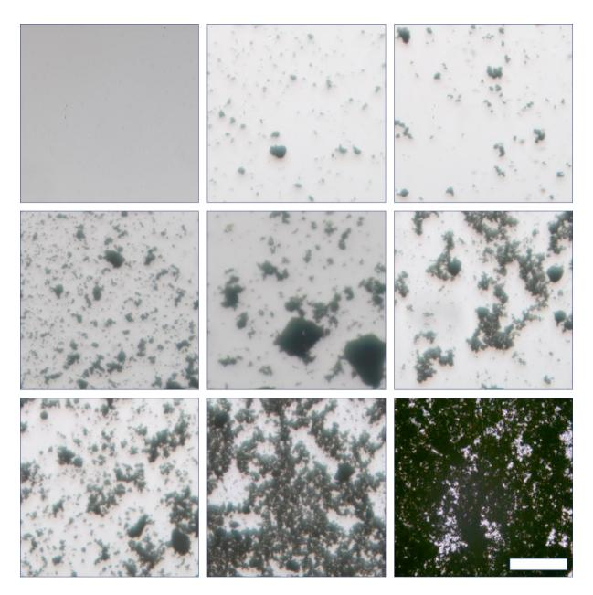
Figure 2. Micrograph 40x magnification for all panes with a common scale bar 50  $\mu m$ . Top left: Resorcinol/formaldehyde/water solution (control). Resorcinol/formaldehyde/water graphene nanoplatelets suspensions with loadings of Top; centre: 0.2 wt.%, right: 0.4 wt.%. Middle; left: 0.8 wt.%, centre: 1.2 wt.%, right: 1.6 wt.%. Bottom; left: 2.0 wt.%, centre: 4.0 wt.%, right: 7.5 wt.%.
