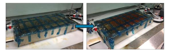
Figure 4. Left: Photograph of RIFT bag containing carbon fiber fabric immediately after infusion of modified carbon aerogel precursor. Right: Photograph of RIFT bag after the curing cycle (3 days later).
