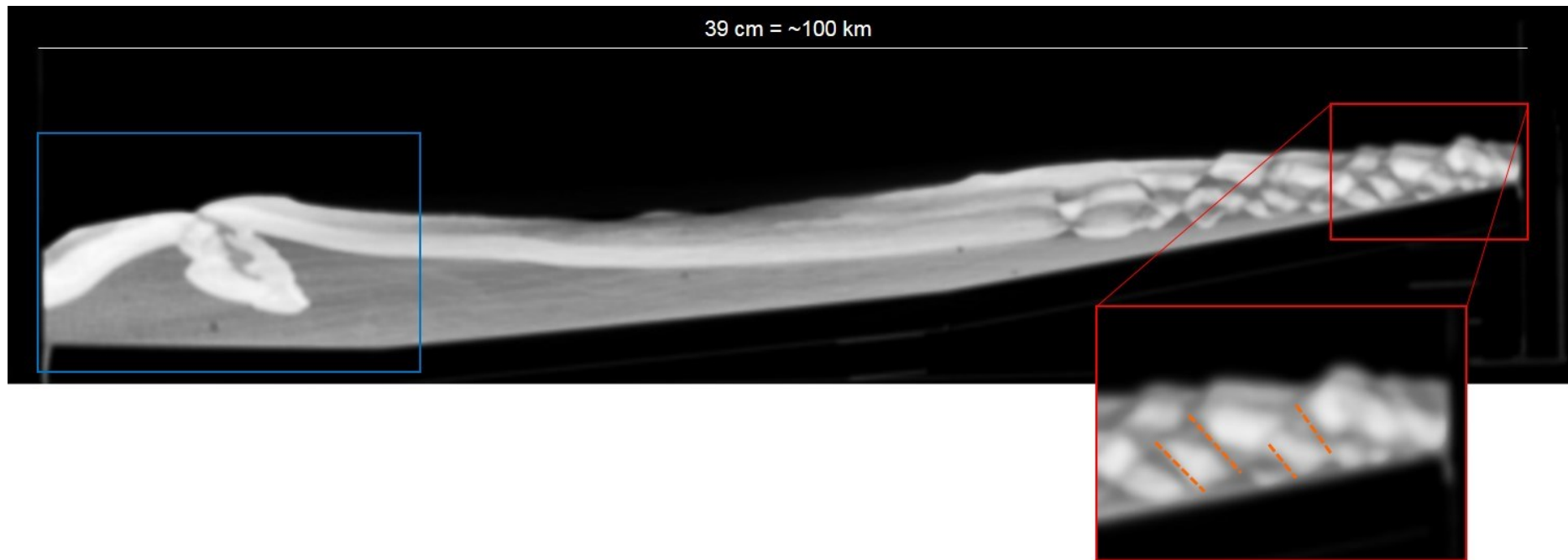
Figure 4.9. Complete cross-section through the analogue model (Evans, pers. comm.). The model is 39 cm in length in real space which corresponds to an analogous passive margin approximately 100 km long. The blue box highlights the basal toe of the ramp, where salt has formed non-monotonic fold structures, which cannot be recreated in the current version of the RRM software prototype. The red box highlights possible antithetic faults (orange dashed lines) in the up-dip section. These faults are difficult to discern at the resolution of the data, and also are difficult to correlate between cross-sections (cf. Figure 4.7). Therefore they were not included in the RRM model
