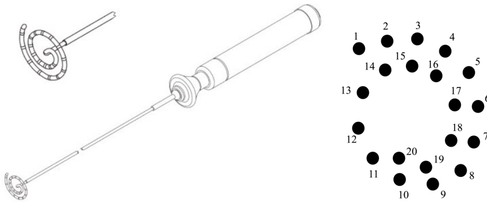
Figure 2.4: (Left) The 7F Inquiry AFocusII catheter with 4F double loop that was used for the acquisition of EGM data. The electrode spacing is 4mm and the loop diameter was 20mm. Adapted from www.cardiovascular.abbott/us/ . (Right) The numbering and arrangement of electrodes on the AFocus II catheter.
