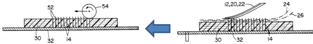
Figure 1.5: Z-pin insertion during cure with thermally decomposable preforms [7]
