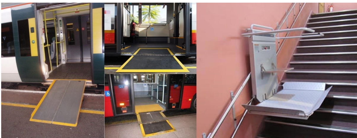
Figure 4.14. A boarding decker and stair lift for wheelchair users
