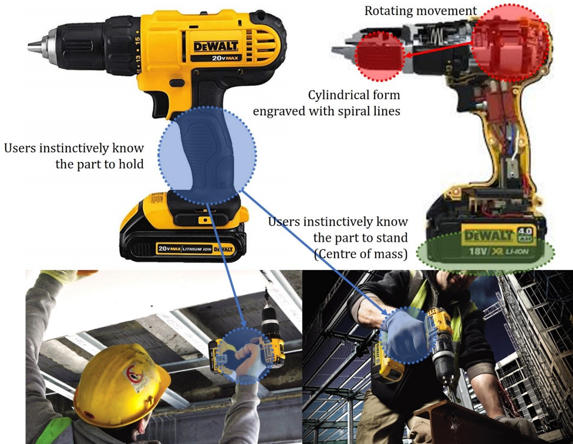
Figure 4.36. Intuitive design of a power drill
