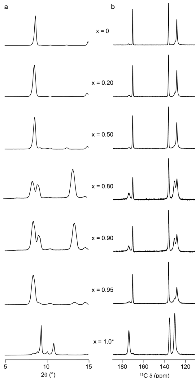
Fig. 2 (a) Partial PXRD patterns and (b) ^{13}\text{C} (14.1 T, 12.5 kHz) CP MAS NMR spectra of calcined (\text{Al}_{1-x}\text{Ga}_x)\text{-MIL-53} for nominal compositions of x = 0, 0.2, 0.5, 0.8, 0.9, 0.95 and 1.0 . *Note that Ga-MIL-53 was calcined at a lower temperature (260 °C) than other materials (300 °C) to prevent framework degradation.
