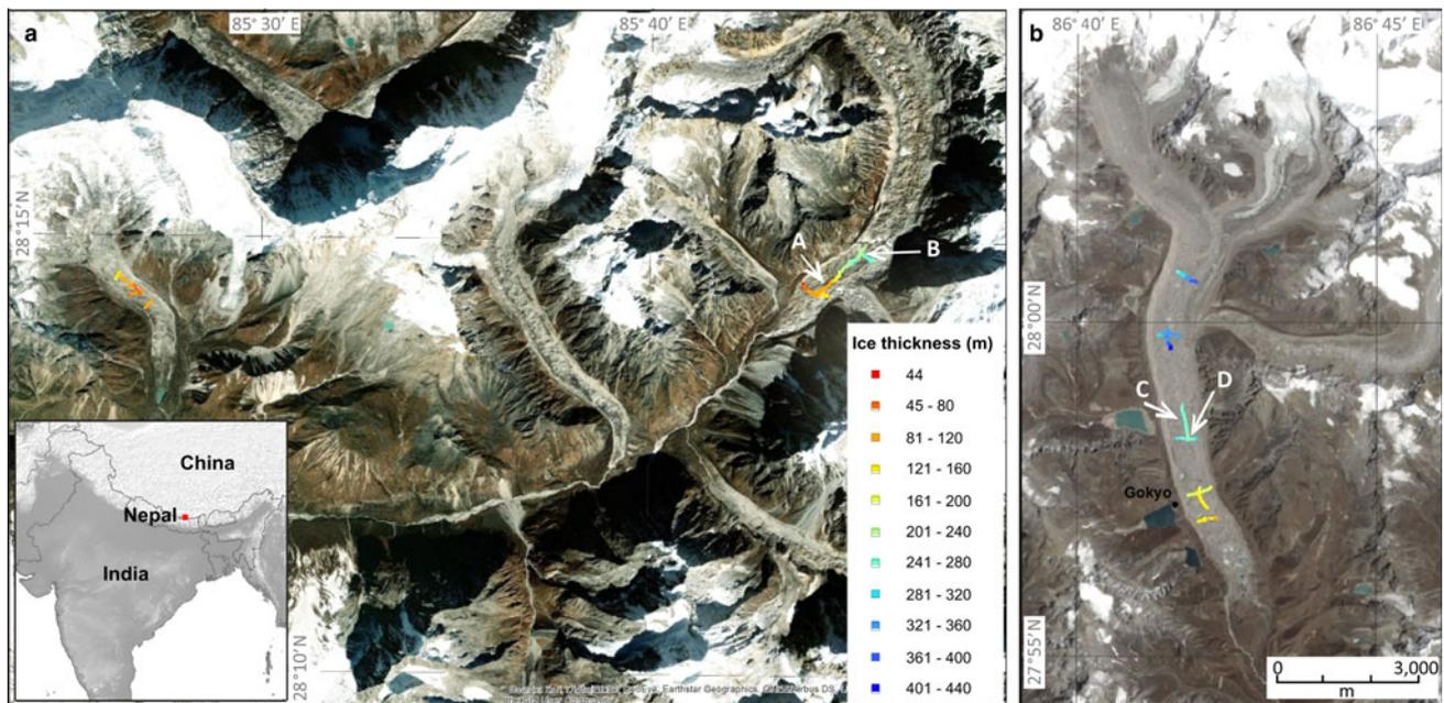
**Fig. 1.** Glacier ice thickness profiling results from glaciers (a) Lirung (left) and Langtang (right), and (b) Ngozumpa. Location of intersecting profiles discussed later are shown by white arrows. Image source: ESRI (GeoEye, DigitalGlobe).
