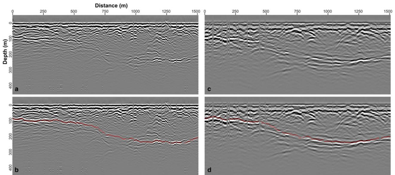
**Fig. 2.** Long-profiles with de-wow, divergence compensation and band-pass filtering from the lower Langtang Glacier (Label A in Fig. 1) at 7 MHz (a) and with bed pick (b), and 3.5 MHz (c) and with bed pick (d).
