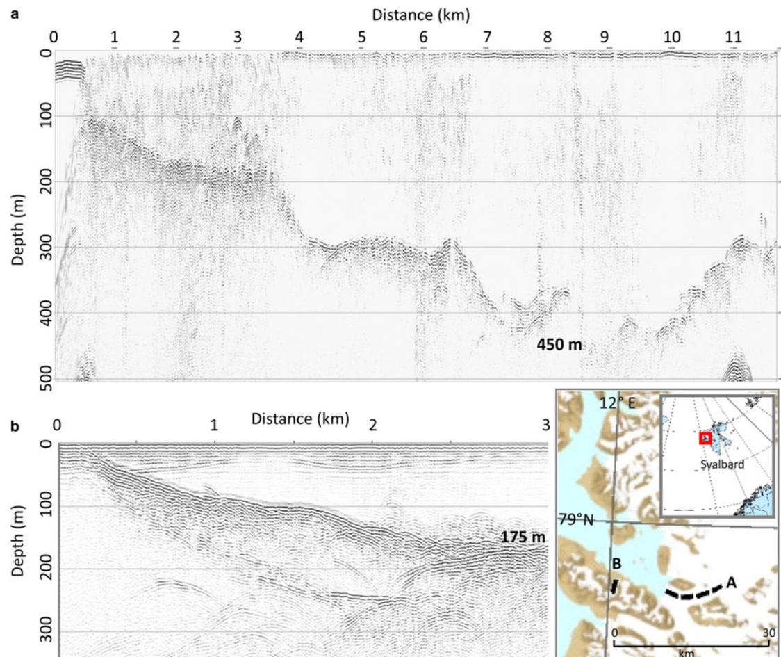
**Fig. 9.** Helicopter-surveyed longitudinal profiles over (a) the lower 13 km of Kronebreen, and (b) the lower 3 km of Midtre Lovenbreen, Svalbard. We calculated depths using a wave speed of  $0.168 \text{ m ns}^{-1}$  in ice. For the heavily crevassed Kronebreen, post-processing with a horizontal averaging filter and a manual gain curve suppressed surface-crevasse clutter by 19 dB. Map data: ESRI.
