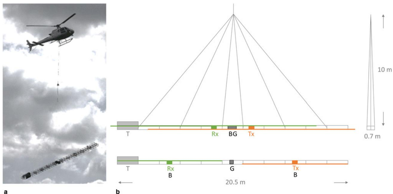
**Fig. 7.** (a) Full-scale airframe prototype. (b) Schematic of radar components, shown configured for 8 MHz (top) and 16 MHz (bottom). Rx and Tx refer to the receiver and transmitter units and antennas, T to the tail, B to battery and G to GPS.
