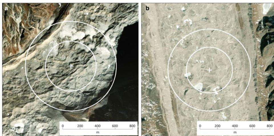
**Fig. 6.** (a) Langtang Glacier and (b) Ngozumpa Glacier radar static-test sites (locations at the AB and CD intersections in Fig. 1). White circles show horizontal ranges that are equivalent to the bed depth for radar propagation speeds through ice (inner circle) and through air (outer circle). Surface features corresponding approximately with the outer circle could provide clutter with a similar time delay as the bed signal. Image source: ESRI (GeoEye, DigitalGlobe).
