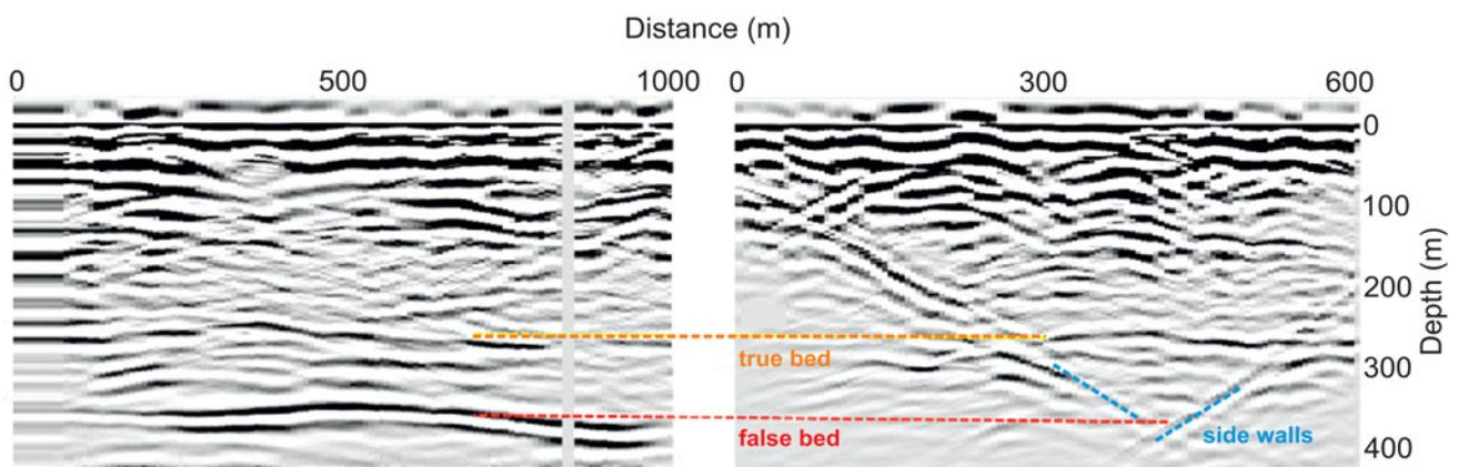
**Fig. 3.** (a) Long-profile (Label C in Fig. 1), and (b) intersecting cross-profile (Label D in Fig. 1) from Ngozumpa Glacier, at 3.5 MHz. The red dashed line indicates a prominent 'false bed', the yellow/orange line, the true bed. The blue dashed lines highlight the trend of the dipping reflectors from the valley walls to the east and west of the glacier.
