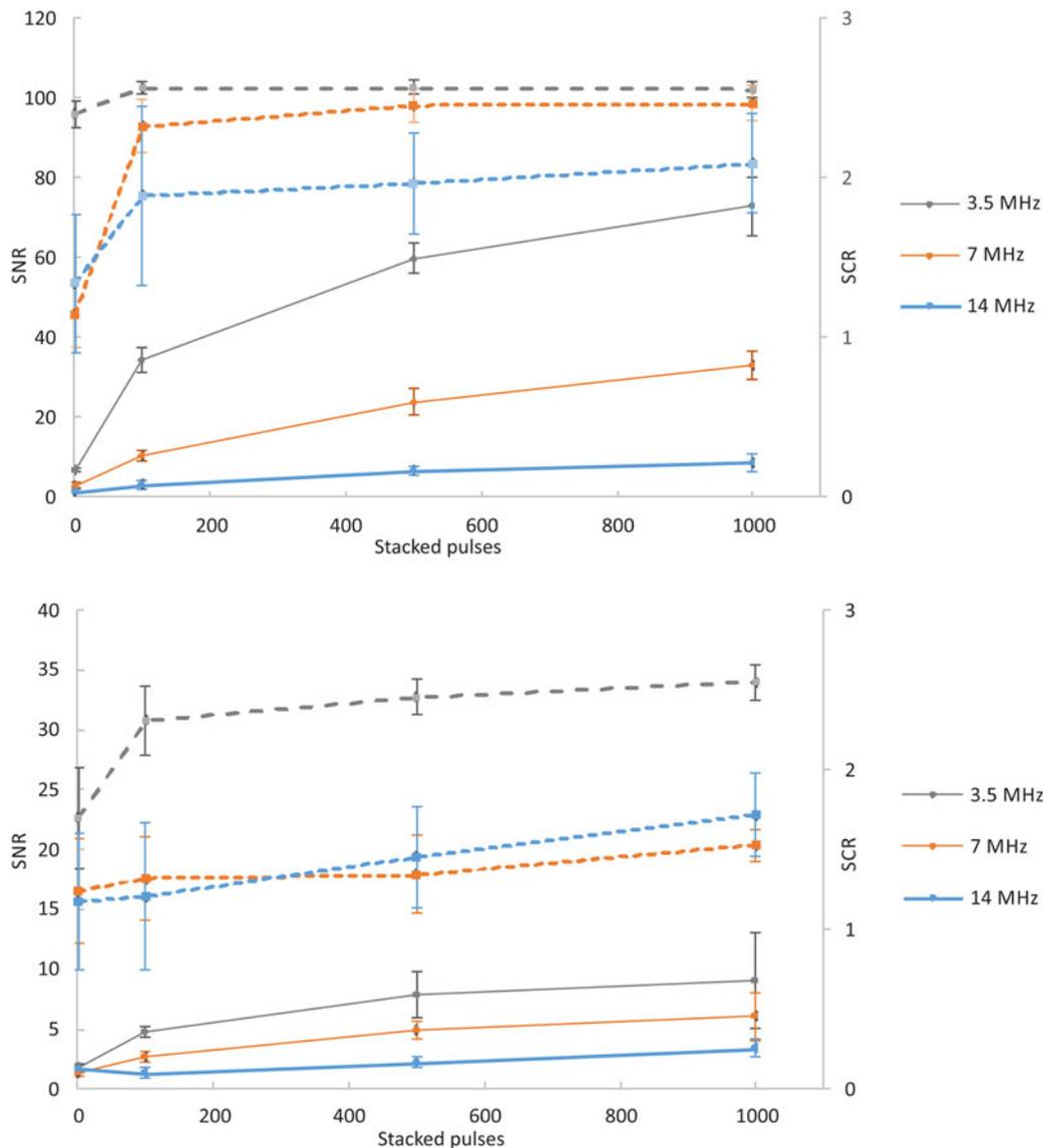
**Fig. 5.** Bed SNR (solid lines, left axis) and bed SCR (dashed lines, right axis) varying with stacking for the three frequencies tested for (a) amplified and (b) unamplified data. Error bars show  $\pm 1$  Std dev. of the ratios measured over 11 repeated stacks for each configuration.
